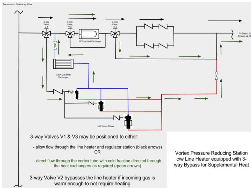
VT has an inlet orifice of a fixed diameter ('no moving parts'), plurality of the VT provides for operations in a broad range of fluctuations of the VPRS inlet flow. Each VT has an upstream control valve (CV) that senses the delivery pressure downstream of the VT. Each CV has a distinct set pressure within the station MAOP, such that each VT begins to supply sequentially as demand increases. Similarly, as demand decreases each VT stops supply sequentially.
